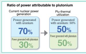
According to the Nuclear Safety Commission of Japan, MOX fuel has characteristics similar to those of uranium fuel under the condition that the ratio of MOX fuel used in the nuclear reactor is one third or less, thus the current safety design and evaluation method can be applied.
