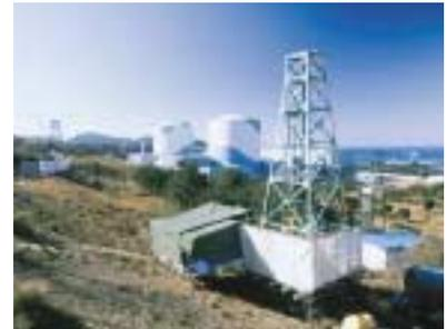
Performed to confirm the rock mass has enough seismic stability as a foundation for a nuclear reactor building.
