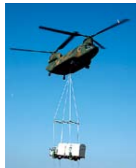
Military helicopter transporting a high-voltage generator truck
