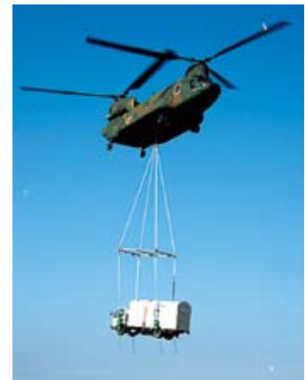
Joint training where a military helicopter transports a Kyushu Electric high-voltage generator trunk
