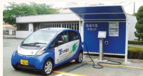
Electric vehicle at a rapid recharging stand
