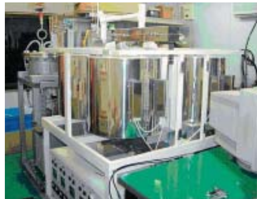
Hydrogen generator with steam electrolysis
