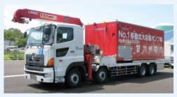
Mobile high-capacity pump truck
