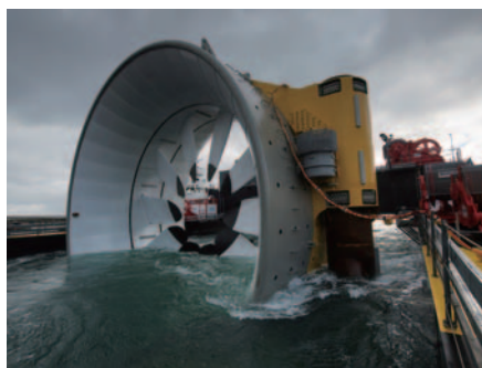
Tidal power electrical generator
