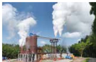
Spouting test at an exploration well to the south of Yamashita Lake
