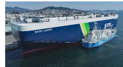
Bunkering vessel (front) supplying LNG fuel to LNG powered vessels (back).
