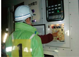
Power supply using a high-voltage generator truck (at night)
