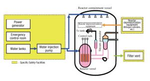
\*1: A facility with functions to prevent damage to the reactor containment vessel in the event that the reactor's core is severely damaged due to the loss of the reactor's cooling ability caused by the deliberate collision of a large aircraft with the reactor's auxiliary building or any other act of terrorism.
