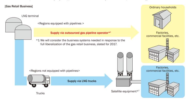
\*2 Facilities for LNG storage, vaporization and delivery
