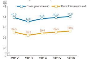
Note: Heating values are calculated on a higher heating value basis (Fiscal Years Ended March 31) In June 2016, operations commenced at Shin-Oita Power Station Unit 3 (Turbine 4), which is the latest combined-cycle unit. In fiscal 2015, as a result of striving to use highly efficient LNG and high rate of operations at coal-fired thermal power plants, we maintained a high rate of total thermal efficiency (at the power transmission end) of 39.6%.
