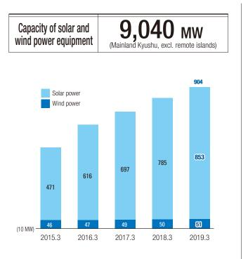
As of the end of March 31, 2019, the capacity of solar and wind power equipment on mainland Kyushu stood at approximately 9,040 MW. As of the end of December 31, 2018, solar and wind power FIT equipment capacity on mainland Kyushu accounts for approximately 17% of the national capacity.
