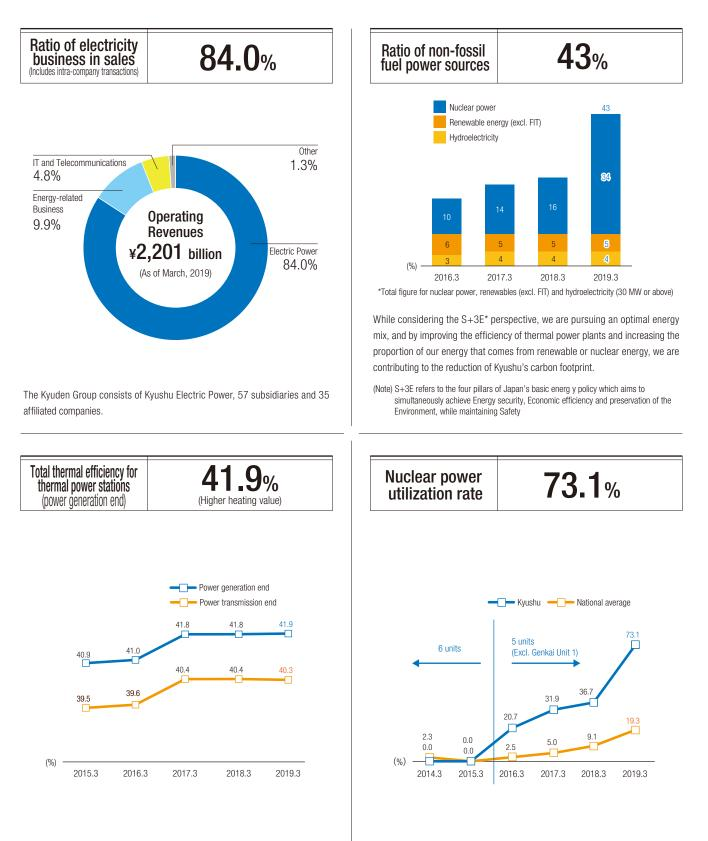
In FY2018, by strictly limited the running of oil-fired thermal power plants, for which thermal efficiency is low, and maximizing operations at high-thermal-efficiency thermal power plants, we maintained our high standard of 41.9% at the power generation end.
