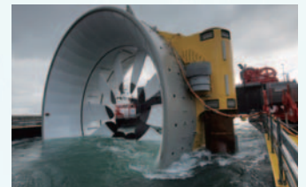
Tidal power electrical generator
