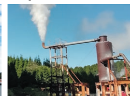
Resource surveys for new geothermal power development sites (Left: drilling to confirm resources; Right: testing to confirm steam capacity)
