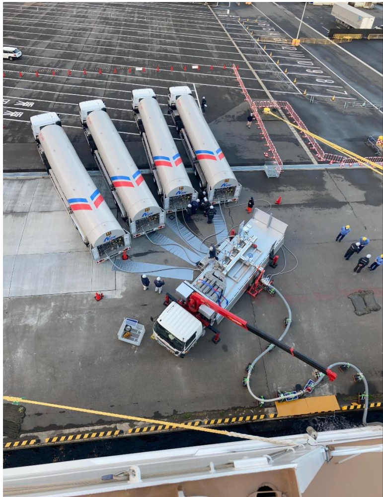
LNG fuel being supplied by four tank trucks and skid
