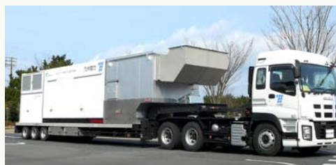
Mobile large-capacity generator (alternate current)
