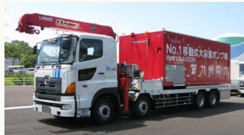
Large-volume pump truck
