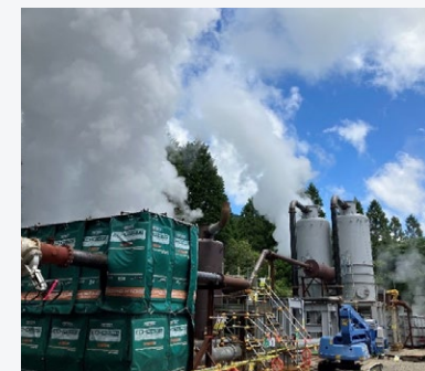
Steam vent test (steam volume survey) at the eastern point of Mt. Waita
