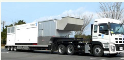
Mobile large-capacity generator (alternate current)
