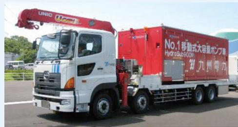
Mobile high-capacity pump truck
