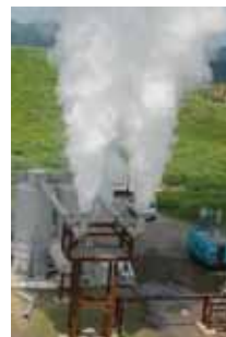
A scene from a well production test at the Sugawara Binary Cycle Power Station
