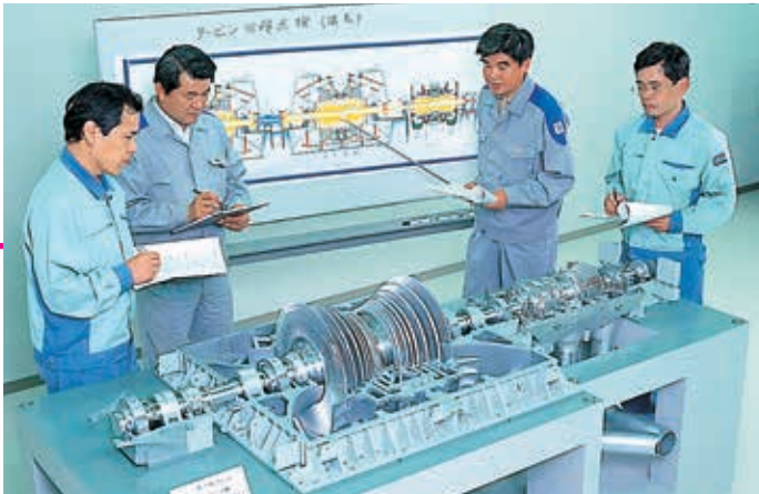
Steam turbine mock-up (1:10 scale) (Lectures on construction and function of steam turbines)
